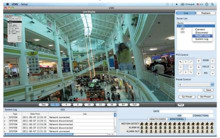
• Health check shows the status of how many cameras are activated, how many HDDs are available, and how many channels are recorded.
